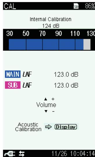
Verify the “Internal Calibration” is displayed in the upper part of the screen.
