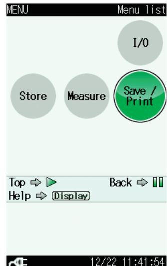
6. Use the  $\Delta$  /  $\nabla$  /  $\triangleleft$  /  $\triangleright$  keys to select [Save/Print] and press the MENU/ENTER key. The save/print screen appears.
